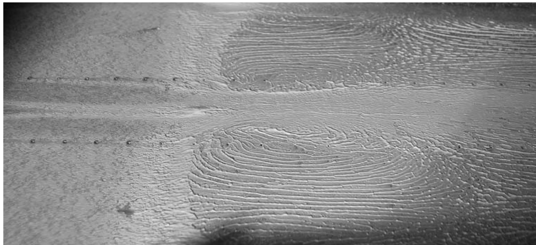
Fig. 18 Visualization of separation: a) baseline, b) 0.4\delta , and c) 0.7\delta .
